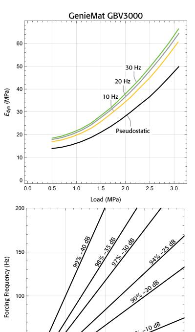
Fig. 3: Applied Load vs Dynamic Modulus
