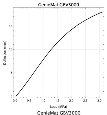
Fig. 1: Applied Load vs Deflection
