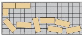
ix. Install the plywood offsetting the seams from the panels and adjacent layers of plywood. Screw the plywood every 12" on center (screw length should not exceed the thickness of the two layers being screwed together).
