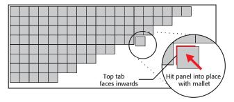
Do not directly hit the edge of the **GenieMat FF** panels with a mallet or hammer. Use a wood block flush with the edge to distribute the load and protect the edges as the panels are hit into place.
