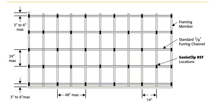
Wall or Ceiling Framing at 16" o.c. **GenieClip RST** at 48" o.c., furring at 24" o.c. 1 or 2 Layers of  $^{5/8}$ " Gypsum Board
