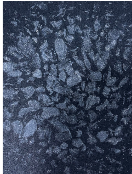
GenieMat RTP contact area with ballast.
