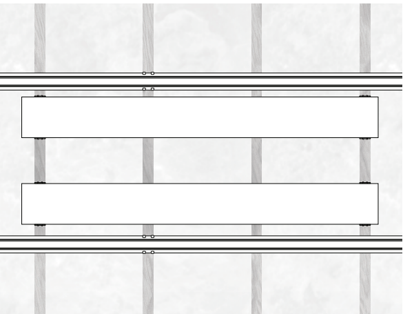
Front view of installed GenieClip Mount and metal stud track.
